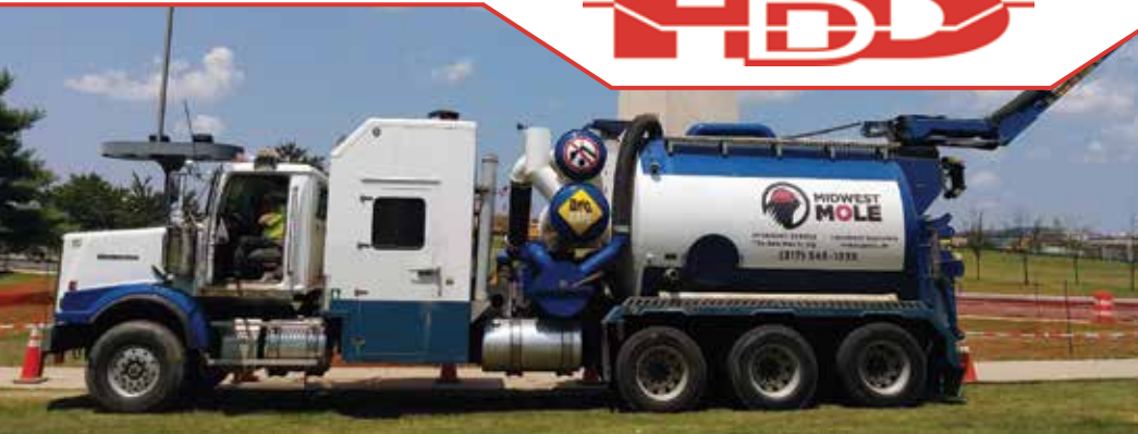
Midwest Mole's Tornado Global Hydrovac hydro excavator works to clean up drilling slurry in front of the Washington Monument.
