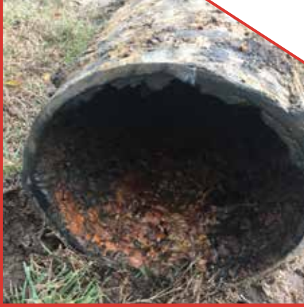
Midwest Mole replaced piping that was 95- to 100-years-old with HDPE. Pipes ranged from 2- to 12-in. in diameter.
